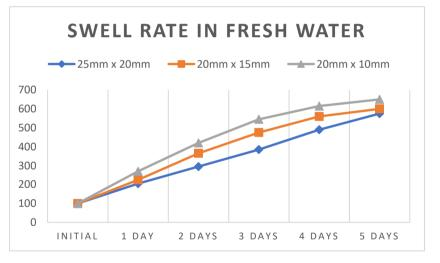
\* Swell rate at 100% indicates original size. Properties are typical under laboratory conditions and do not constitute specification.
